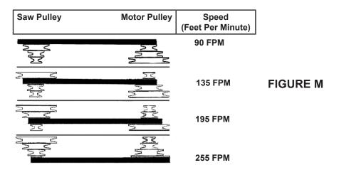
4. Verify belt tension by pressing the belt between the pulleys. Deflection should be about 3.8". In time, the belt will stretch and loose its tension. Loosen the Hex Nut (302) and back off the Belt Tension Limiter Bolt (301). Turn the Belt Tension Limiter Bolt (301) against the Motor Mount Bracket (307) and tighten the Hex Nut (302).
